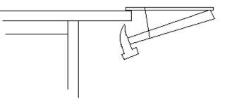
This works because the center of mass (somewhere near the hammerhead) is under the supporting end of the ruler on the tabletop. It looks impressive because the majority of the ruler and handle is suspended off the edge of the table.
