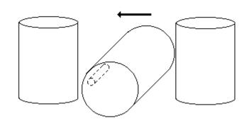
of their observations. Then perform the ultimate experiment and take the lid off the can that has rolled back and forth and show them how things have worked. Inside have an AAA battery (thus battery operated) glued to one side. The teacher has simply set the can down so that the battery inside has made the can roll in a desired direction.
